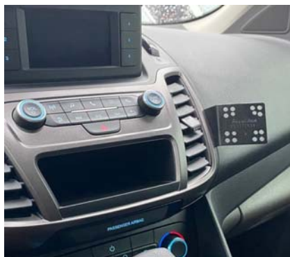
InDash installed upper location
