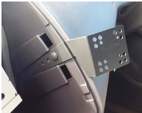
InDash installed upper location
