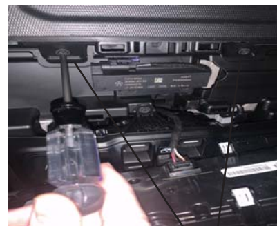
Screen bezel screw locations.
