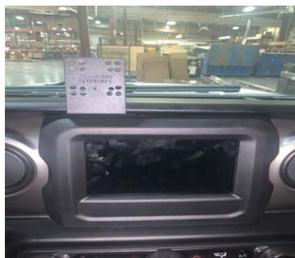
InDash Mount Installed
