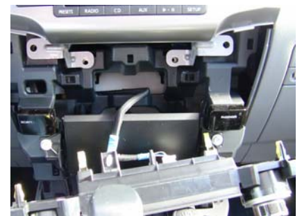
Climate Control removed showing radio screws location
